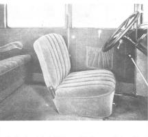
The driver's seat is fitted with the new quick adjustment mechanism and is easi regulated, even when occupied, to accommodate the long or short reach. Mothers we because of small children, brefer the two-door type athreciate this convenient featu
